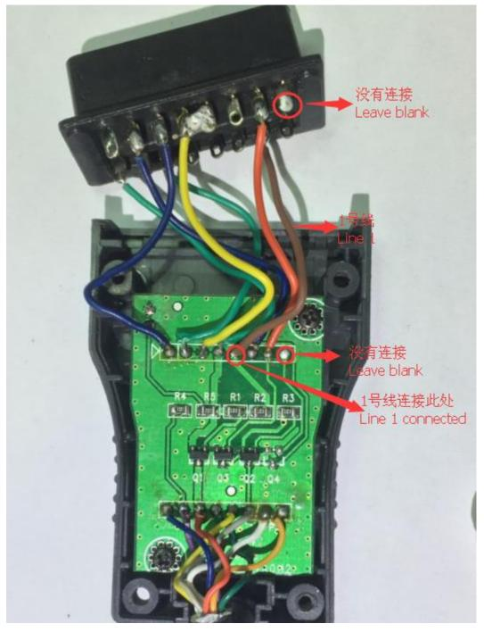
(PICTURE 14. 3) CAS PLUG works on VVDI2 (modified)
